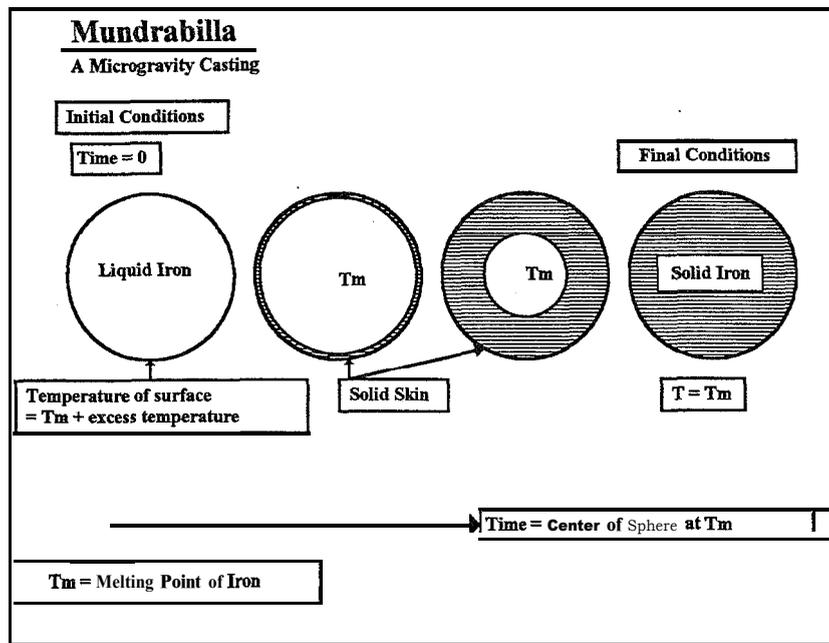
Figure 7: A typical nickel-iron meteorite modeled as a multi-kilogram ferrous liquid sphere solidifying under microgravity conditions in outer space.
