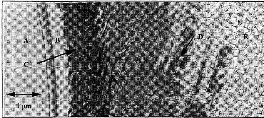
Figure 4: Typical meteoritic delta ferrite-austenite-plessite region. Region A is delta ferrite/kamacite; B is austenite/taenite; C-D-E is classically described as plessite.
