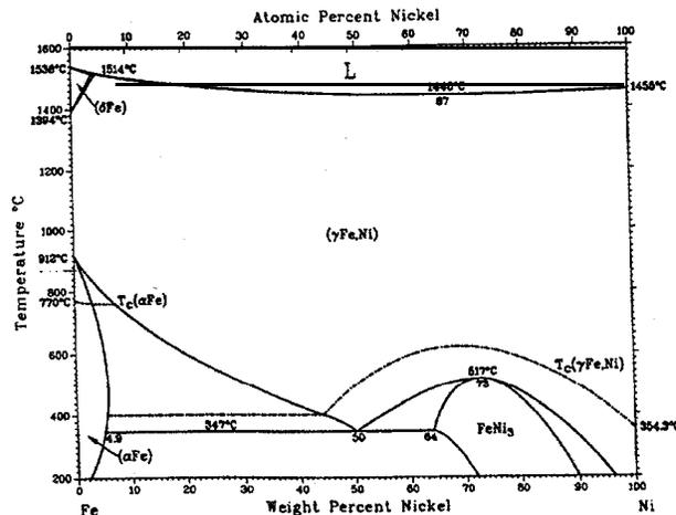
Figure 3 - Fe-Ni phase diagram (6).
