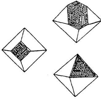
Figure 1a: Schematic of Widmanstätten structure (3).
