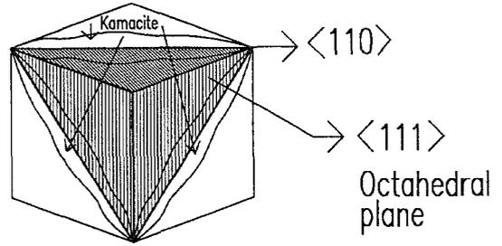
Figure 1b: Widmanstätten kamacite/delta ferrite growth in the <110> direction defines a <111> octahedral plane.
