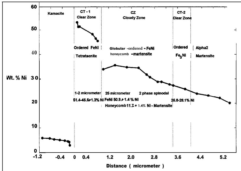
Figure 5: Schematic microprobe trace of **typical** nickel-iron meteorite phase regions. After reference (4).
