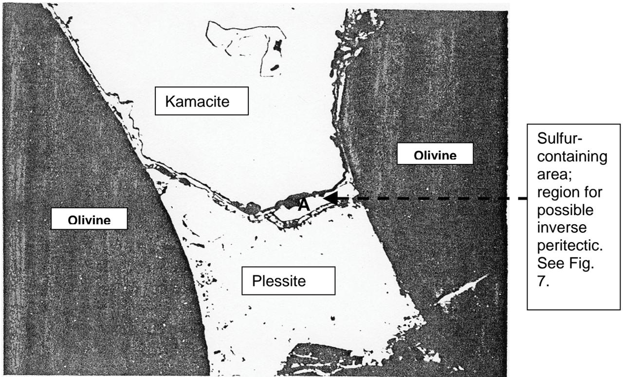
Figure 6 Area of Springwater pallasite (stony iron meteorite) subjected to EDAX analysis (50 x). See Fig. 7 for x-ray analysis of region A.
