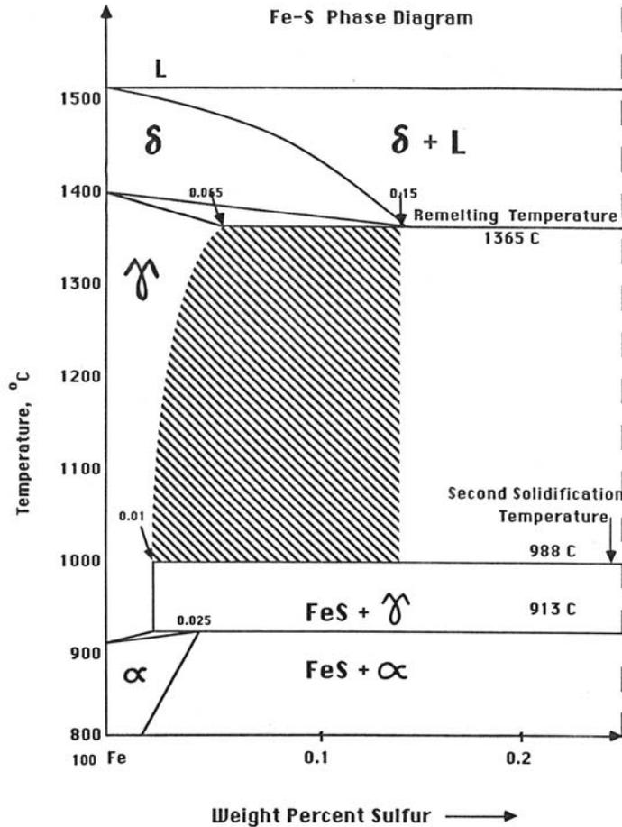
Fig. 5 Hatched area shows the range of temperature and composition over which liquid can occur for a second time, due to the inverse peritectic phase transformation. Liquid can reappear over a temperature range of 400C and over an order of magnitude in sulfur composition.
