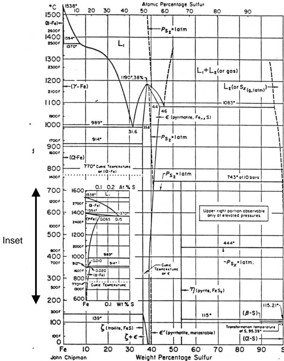
Fig. 2 The Fe-S phase diagram; American Society for Metals "Handbook." Inset is low sulfur region up to 0.2 w/o sulfur, 600-1600C, containing inverse peritectic transformation.
